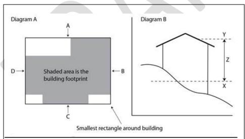
Diagram A: A through D represent the elevation midpoints for each side of the Building.
